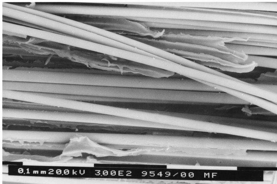
Figure 10 SEM photo of fracture surface of flexural test of air cooled sample.
